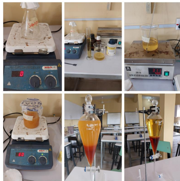
Plate 3.2: Extracted sandbox oil undergoing transesterification to obtain sandbox methyl ester and Glycerol
