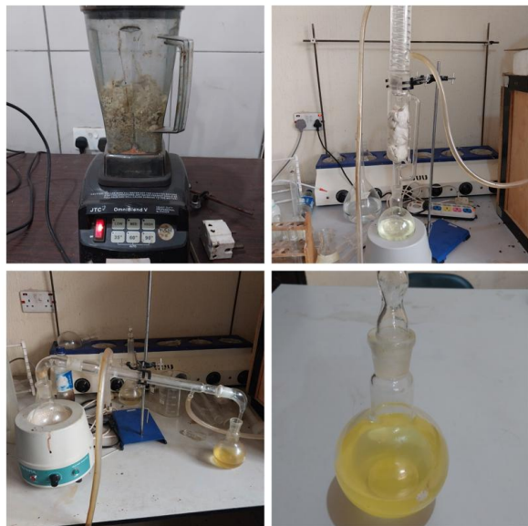
Plate 2.1 Sample preparation and Solvent Extraction of Sandbox seed oil
