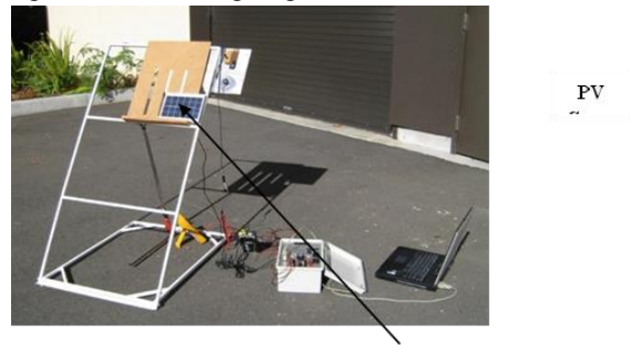
Sample Figure 3 Custom-built by SERC IVCT For testing smaller modules I_{sc} \leq 2A
