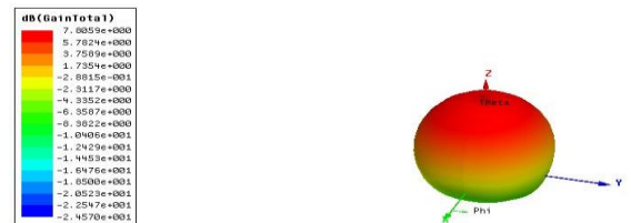
Figure 5: Gain plot for rectangular MPA
