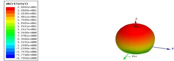
Figure 4: Radiation pattern in 3D of Rectangular MPA
