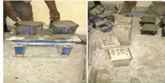
Figure 1: Casting of concrete specimen
