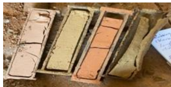
Plate 6: Clay Samples after undergoing Shrinkage limit
