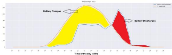
Fig.11. Battery Charging and Discharging Time periods
