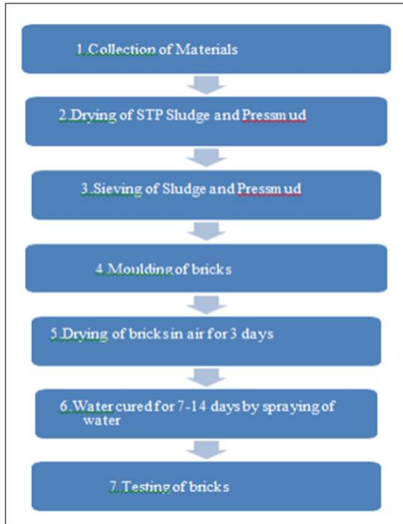
Fig. Manufacturing process of STP mud bricks
