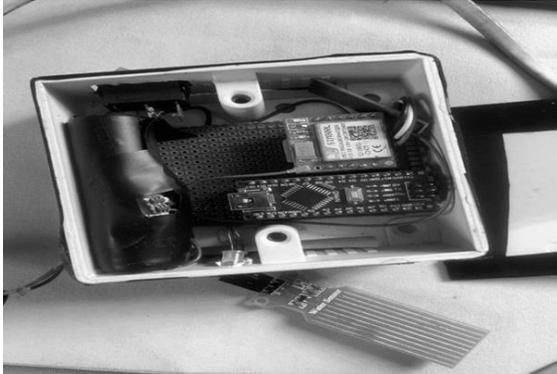
Plate 3: Circuit design on Veroboard
