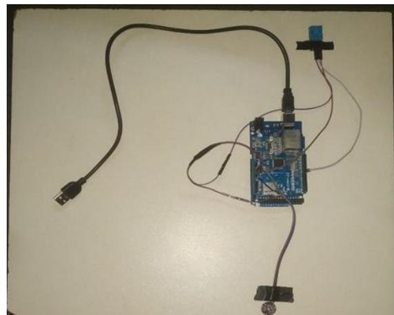
Fig.5 Hard ware connection of Health Monitoring system with Arduino and Sensors
