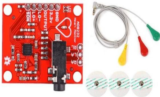
Fig.3 AD8232 ECG Sensor
