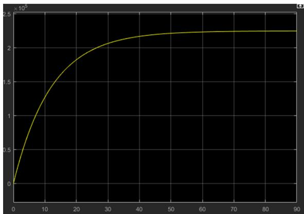
Figure 4.3: Fuzzy controller-based kiln response
