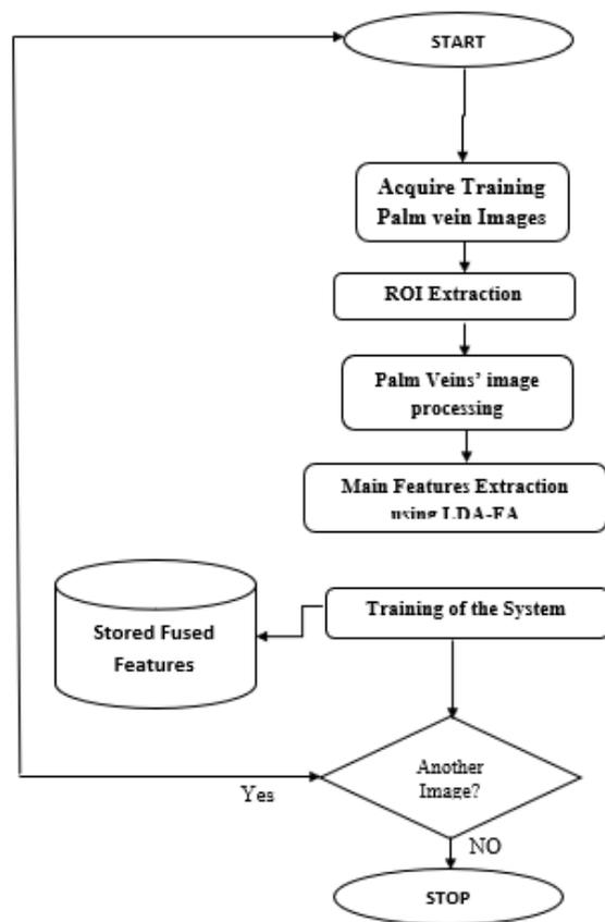
Figure 3.3: Flowchart of Training Stage of the Developed System
