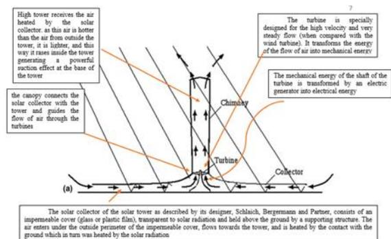
Figure 1. Solar Updraft Tower Principle (Shadi Kalasha, Wajih Naimeh, Salman Ajib, 2014)
