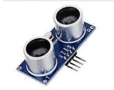
Figure 2: Ultrasonic sensor
