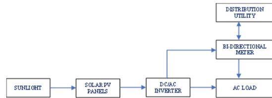
Figure 2: Block Diagram of a Grid-Tied PV System
