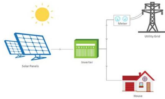
Figure 1: Grid-Tied PV System Setup
