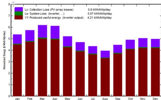
Figure 9: Normalized Production Diagram
