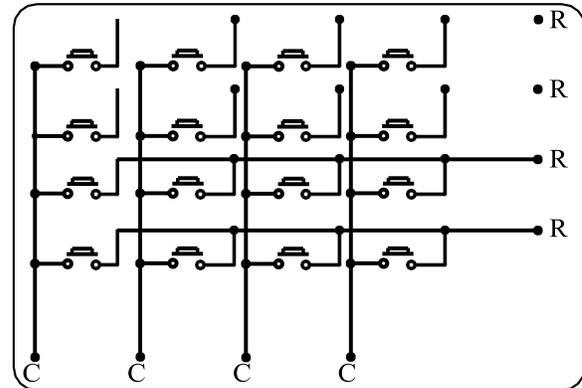
Figure 3: Internal structure of 4X4 keypad module
