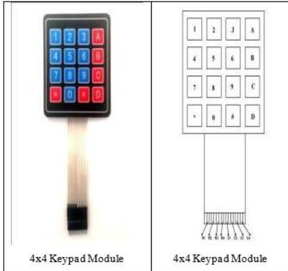
Figure 2: 4x4 Keypad Module
