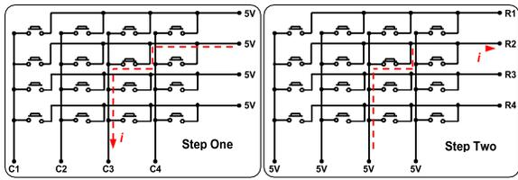
Figure 4: 4X4 keypad module button determination steps
