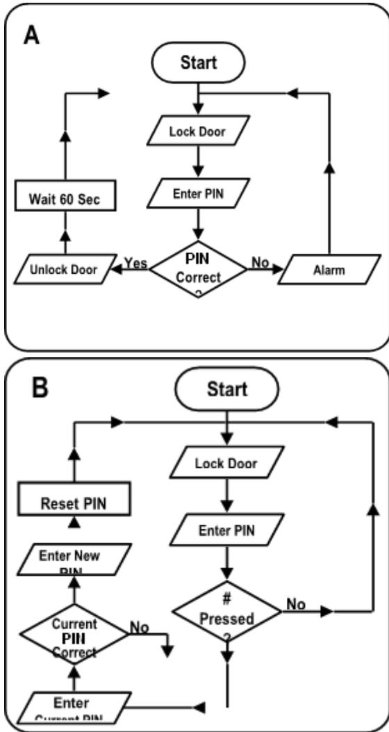
Figure 5: (A) System locking and unlocking flow chart (B) System PIN reset flow chart
