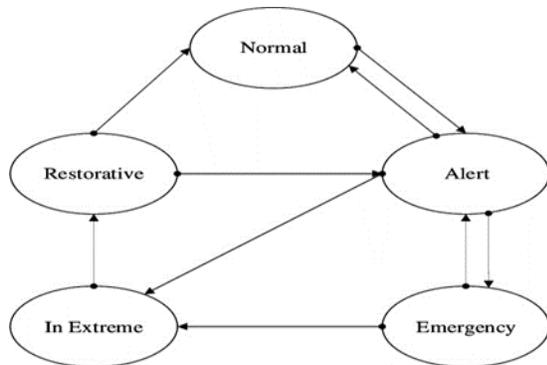
Figure 1 Operating states of power system
