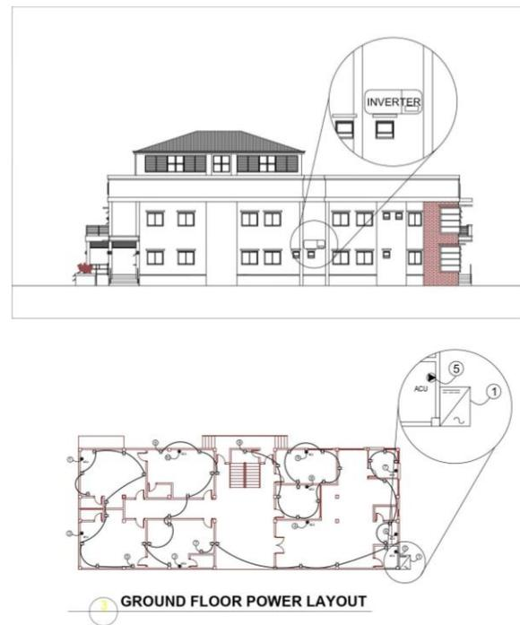
The inverter is located on the east wing of the administrative building, parallel to the generator. The inverter should be covered to protect it from weather conditions. The system's average daily demand is 45.77 kW, with an extra 25% future load of 57.2127 kW according to market availability the inverter size is 60 kW. The On-Grid Three Phase Inverter consists of a maximum input DC voltage of 1100V, maximum input DC of 26 A per Maximum Power Point Tracking
