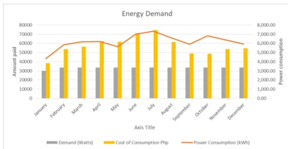
The Total kWh per month is 6,179.33. While the Total kWh per day is 205.98. The total peak sun hours is 45.77 kWh and for the Future loads is 57.2125 kWh.
