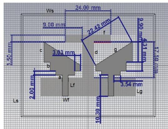
Figure 1: Top view of proposed antenna
