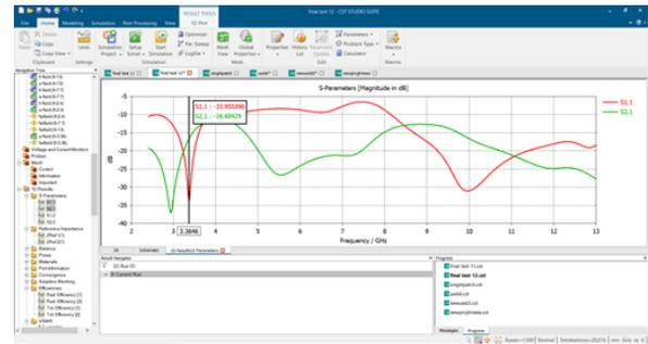
Figure 3: Simulated S-Parameters, to illustrate the effect of change in ground plane.
