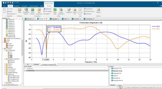
Figure 5: S-Parameters of the designed UWB-MIMO antenna.
