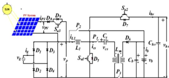
Fig. 3. Configuration of the proposed power conversion system.
