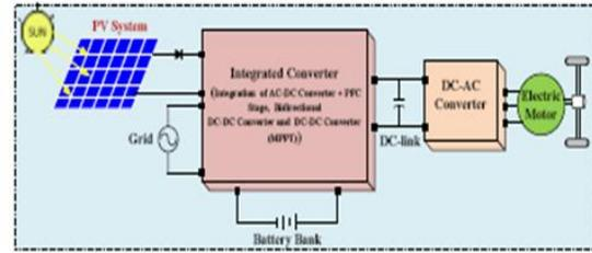
Fig. 4. Block diagram of the proposed system.
