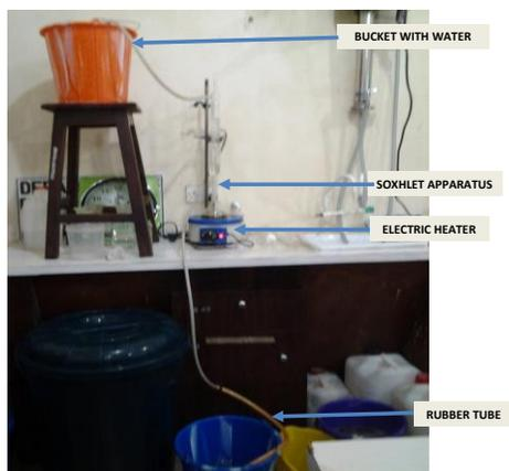
Figure 3.4: Solvent Extraction Method II
