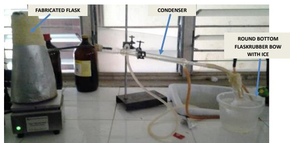
Figure 3.3: Steam Distillation
