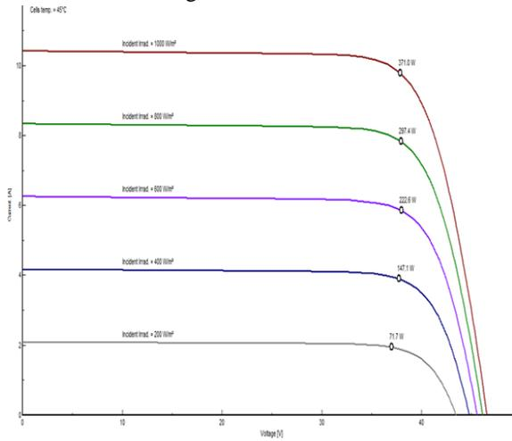
Figure 4.4: I-V Characteristics of the Solar Panel Used at Constant Temperature
