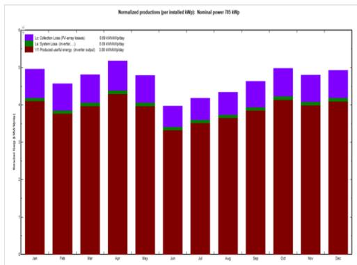
Figure 4.2: Normalized Production (Per kWp)
