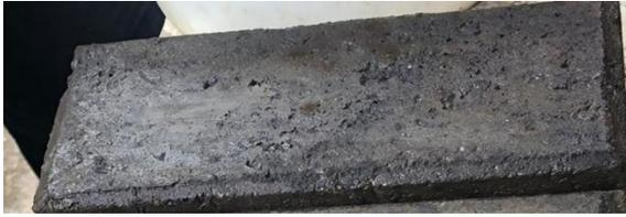
Fig 3.1 Porous Surface of the PET: Sand Blend
