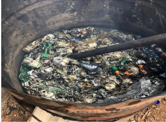
Figure 2.4: Melting PET Bottles
