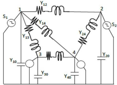
Fig. 2: One-line diagram of a 4-bus system
