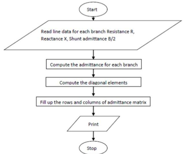
Fig. 3: Flow chart for computing the admittance matrix
