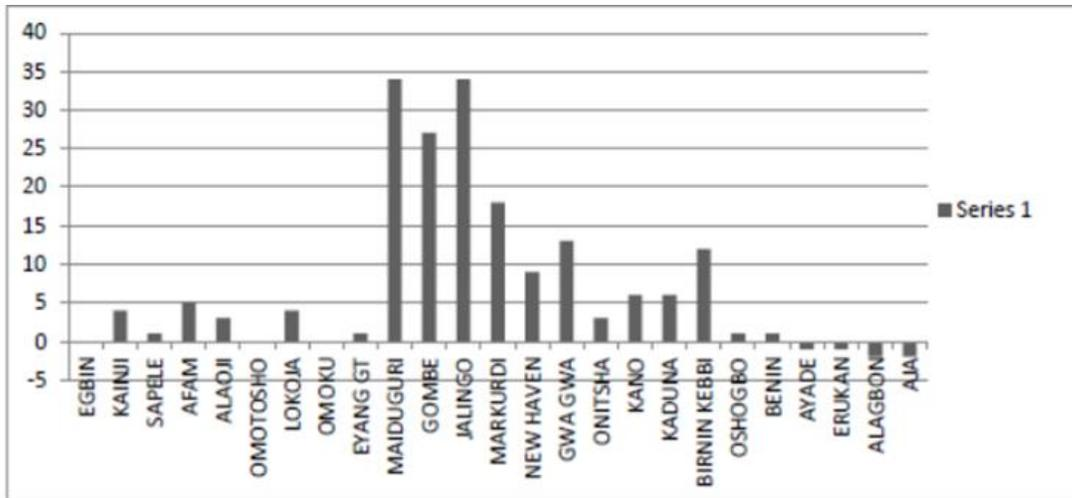
Fig. 5: Voltage Violation Profile before Compensation (+10% and -15% limit)
