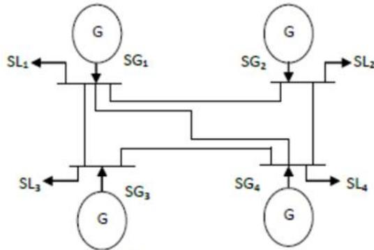
Fig. 1: One line diagram of a 4-bus system
