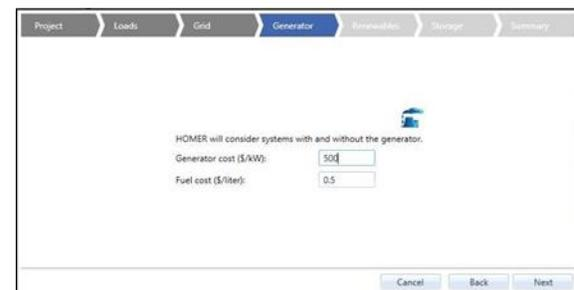
Figure 4.4: Generator settings for the system simulation.
