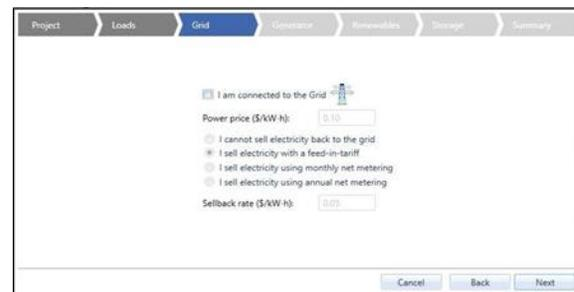
Figure 4.3: Grid settings for the system simulation.
