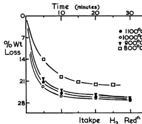
Figure 6: Isothermal mass- change data for H<sub>2</sub> reduction of Itakpe ore
