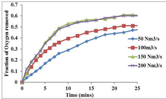
Figure 10: Fraction of Oxygen removed at different Reducing gas Flow rates
