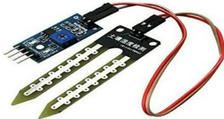
The 2 copper leads act like the sensor probes. They are dipped into the specimen of soil whose moisture
