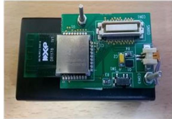
Figure 2.0 Radio module
