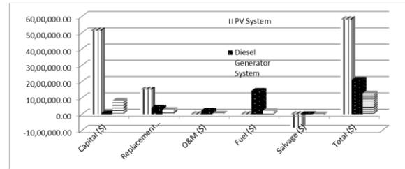
Figure 3: Comparison of system cost (Homer Simulation Tool)
