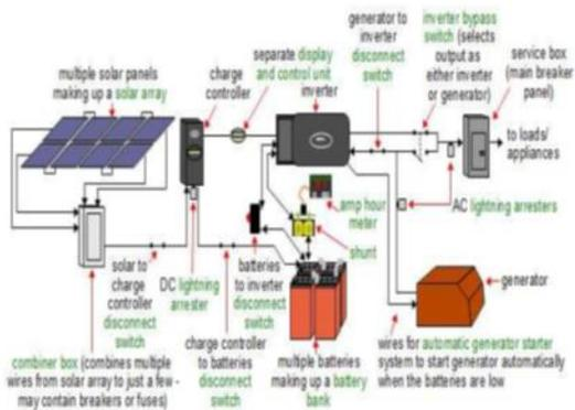
Figure 2: Solar power system structure and working principle [3]
