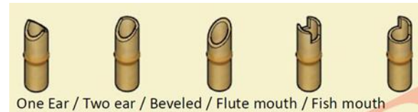
Figure 2 – Types of cut on bamboo
