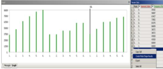
An interesting alternative to this view is to see the sorted frequency spectrum. You may review this by setting the X-Axis to Frequency on any of the Total Deformation results in each modal analysis:
