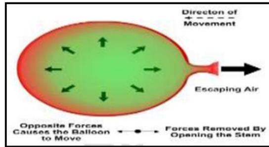
Figure: 5. Balloon example of jet propulsion theory
