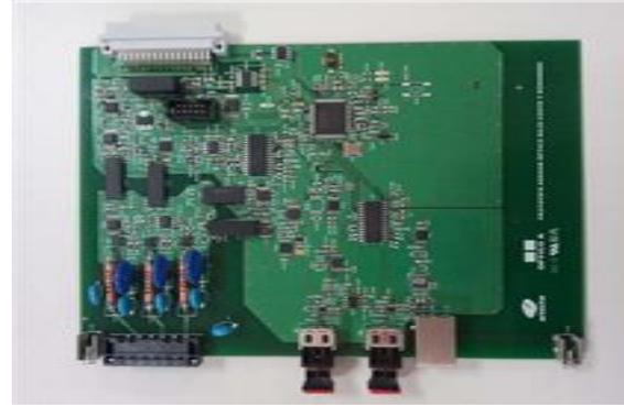
Figure 5. Custom electronic hardware for the acquisition of the current sensor signals.
