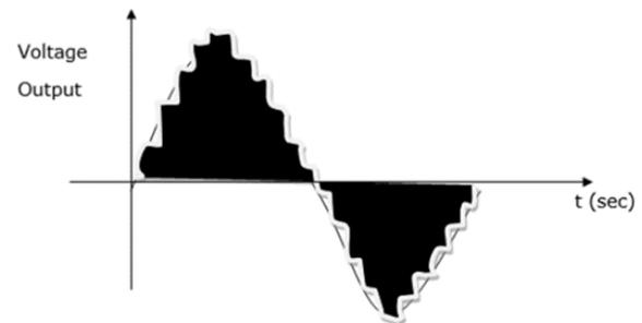
PWM (pulse width modulation) or PDM (pulse-duration modulation) is a technique for decreasing the average power produced by an electrical signal by splitting it up into discrete parts. By rapidly flipping the switch between supply and load on and off, the average value of voltage (and current) provided to the
