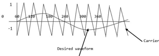
$A_m$  denotes the sinusoidal amplitude, while  $A_c$  denotes the carrier triangle. The modulating index  $m$  is equal to  $A_m/A_c$  for sinusoidal PWM.
