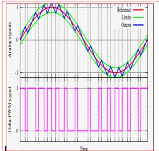
There are three types of pulse-width modulation (PWM):
