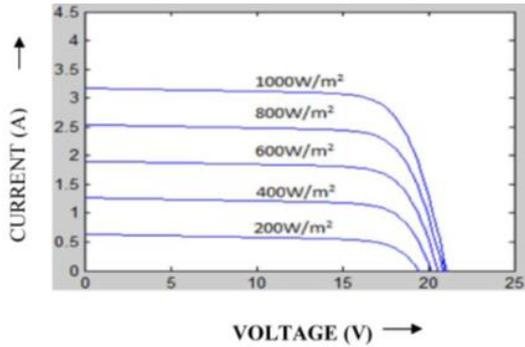
Fig. 2: Current vs Voltage characteristics of PV array
