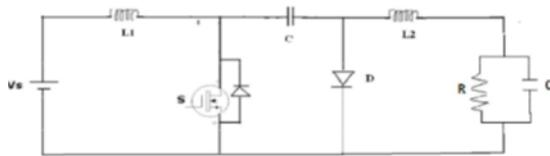
Fig 7: Schematic diagram of cuk converter
