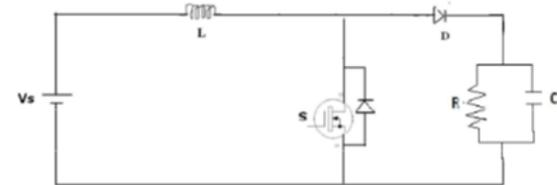
Fig 5: Schematic diagram of boost converter
