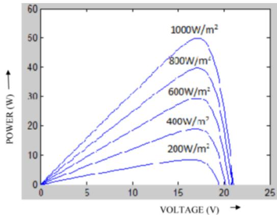
Fig 3: Power vs Voltage characteristics of PV array
