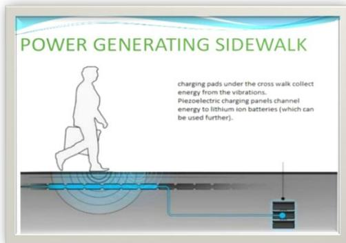
The maximum of 2mW energy is generated and charges 40mAH button cell battery in 1 hour. As the mob farmstead won't work in the home, the power that will be required to light 15 LED lights for 1 second will be produced from a single human step.
