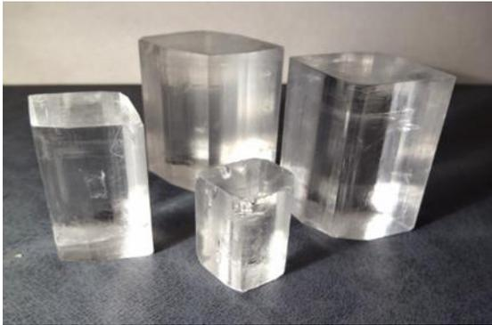
When this crystal is placed in electric field exposed first to a shearing stress. So, in the event of plates cut with all edges that are parallel to the axes, the expected type in an alternating field is shear vibration. Although the possibility of longitudinal vibration is not eliminated through elastic reactions. Rochelle salt crystal can also be cut into plates in such a way to show shrinkage and restaurant extensions in directions perpendicular to field of electricity.
