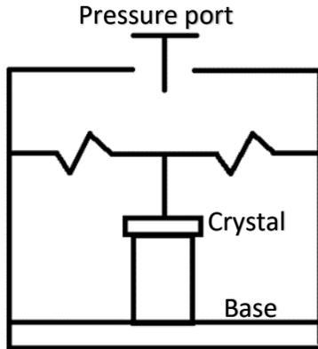
Between two metal plates, the piezoelectric crystal is deposited. On the metal plates the mechanical pressure will be applied that efforts the electric charge with in the crystal off-balance.
