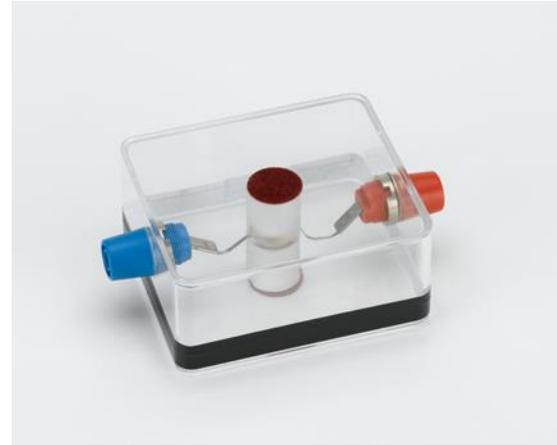
This Rochelle salt was the first material that was discovered by Valasek. He found the ferroelectric phenomenon in Rochelle salt in 1921. From this he also introduced curie temperature and curie point of ferroelectric. There are some differences between Rochelle salt and quartz.
