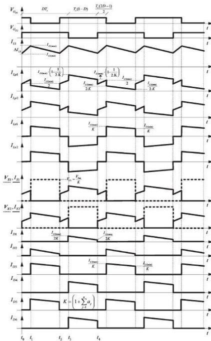
FIG 3: Theoretical waveforms for the proposed converter
