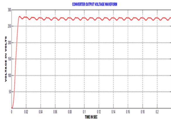
iii. SEPIC CONVERTER OUTPUT VOLTAGE WAVEFORM
