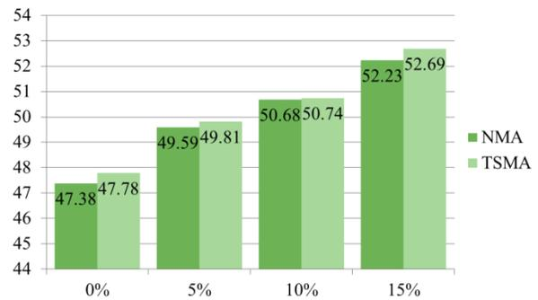
husk ash can be used as a provides the reduction in burden on land fill disposing and environmental pollution. The results shows that the good strength addition of fly ash and rice husk ash exhibits increase in compressive strength up to 15% replacement. Fly ash and rice husk ash can be used as binding material to partial replacement for rapid hardening cement. Recycled course aggregate can be used as coarse aggregate to 25% constantly replacing, this result in saving of natural aggregate.
