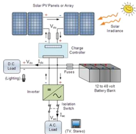
Figure 1. Components of Stand –Alone PV System
