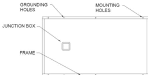
Fig.6. Back Side of Module
