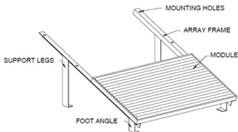
Fig.8. Basic Rack or Standoff Module Mounting Structure
