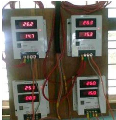
Fig.4. Charging Voltage and Current of Each Controller
