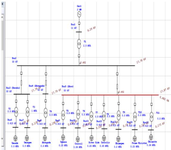
Figure 3: Pre-Fault Simulation on 33KV Distribution Feeder with Single Line to Ground Fault at Bus 3 (Abor Community).
