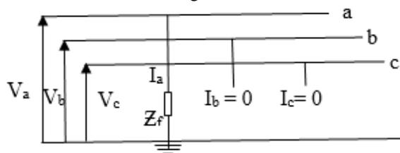
Figure 5: Single Line to Ground Fault
