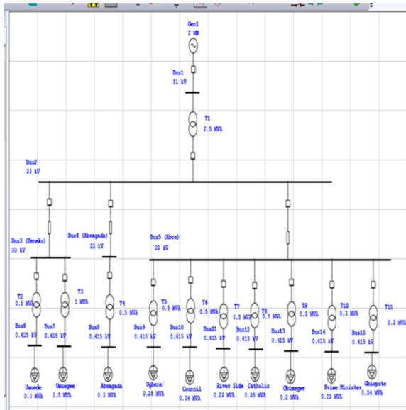
Figure 6: The Post- Fault 33KV Distribution Network for Beneku, Abragada and Abor community in Delta State, Nigeria.
