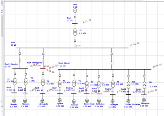
Figure 2: Pre-Fault Simulation on 33KV Distribution Feeder with Single Line to Ground Fault at Bus 4 (Abragada Community).
