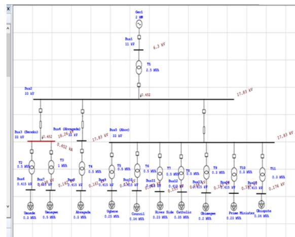
Figure 1: Pre-Fault Simulation on 33KV Distribution Feeder with Single Line to round Fault at Bus 3 (Beneku Community).
