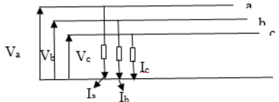
Figure 4: Distribution Network with Unbalanced Three-Phase Fault
