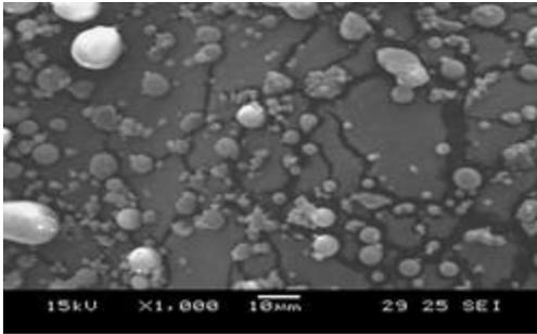
Fig. 1 SEM of Fly ash
