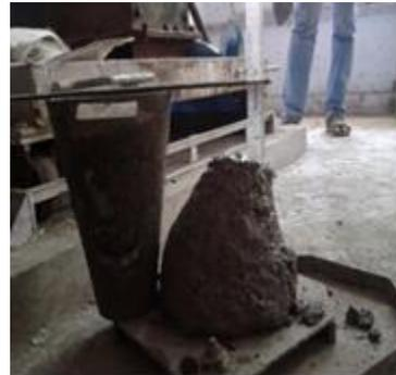
Figure 5 Measuring of Slump
