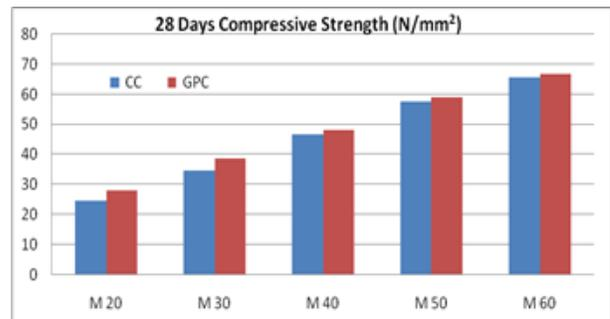
Figure 9 Compressive Strength of CC and GPC Cubes
