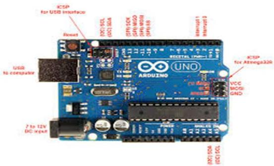
The Arduino Uno is a microcontroller board based on the ATmega328. It has 14 digital input/output pins (of which 6 can be used as PWM outputs), 6 analog inputs, a 16 MHz ceramic resonator, a USB connection, a power jack, an ICSP header, and a reset button. It
