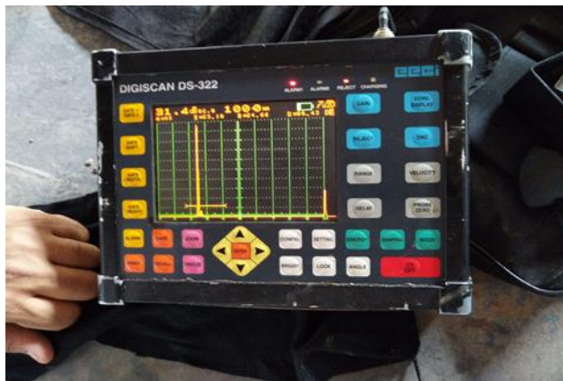
Figure 3 Image: - Ultrasonic testing Machine
