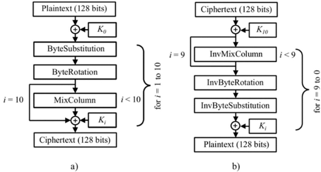
Fig1: Block diagram of cipher Rijndael (a) encryption algorithm (b) Standard decryption algorithm
