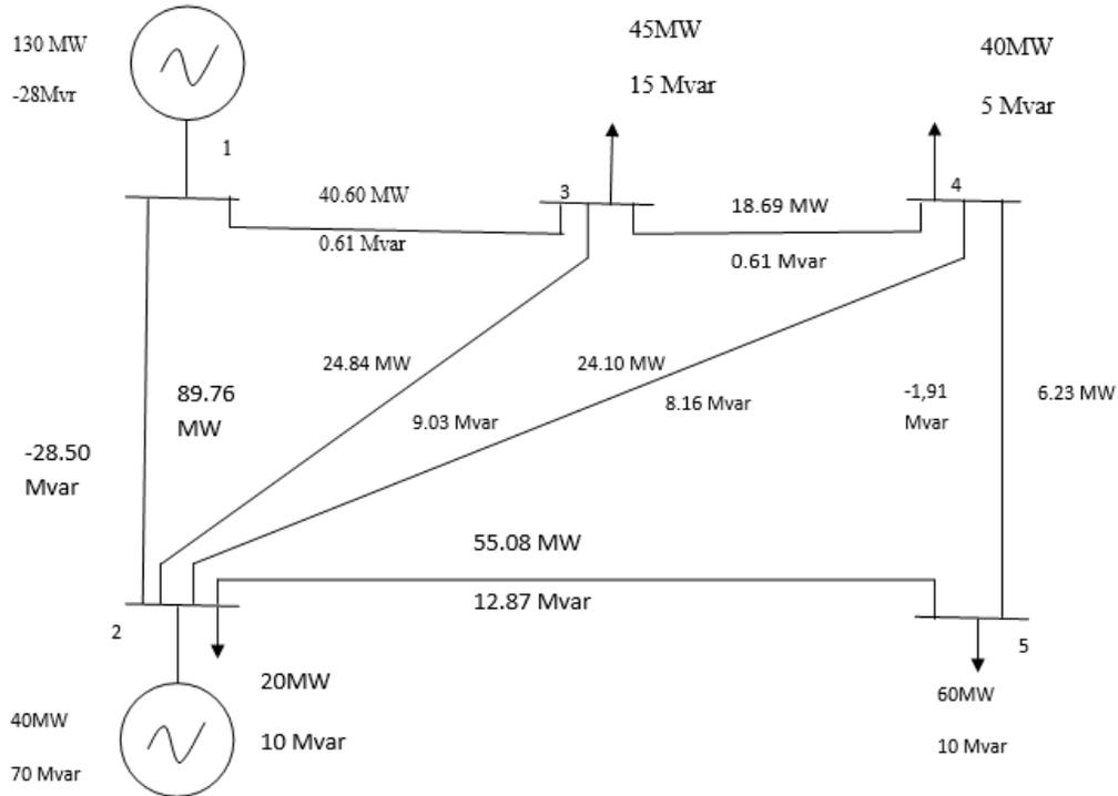
Fig. 4 Transmission margins without TCSC
