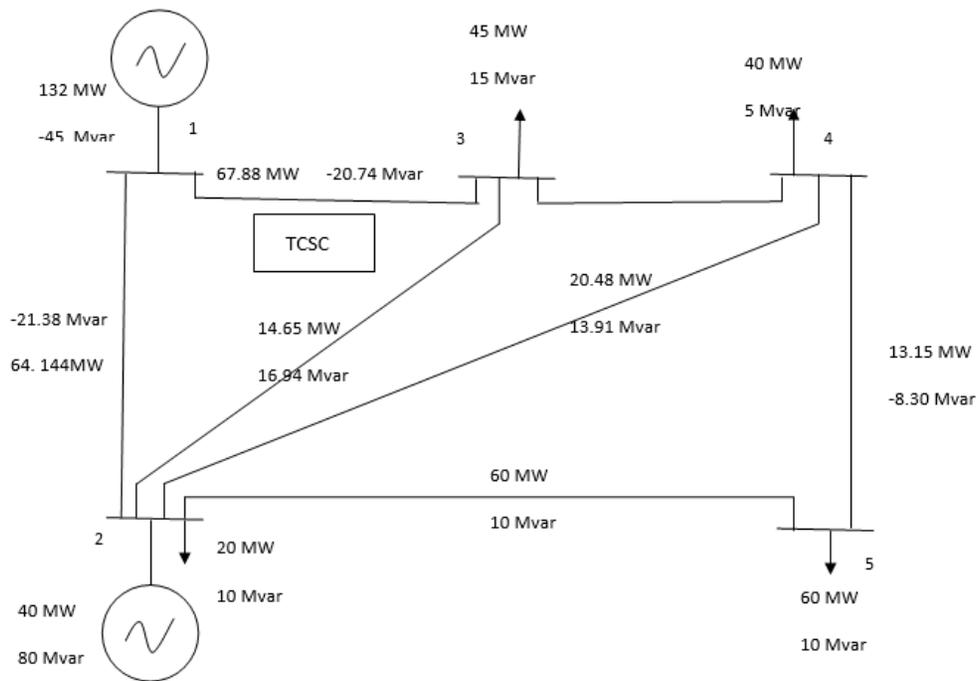
Fig.5 Transmission margins with TCSC
