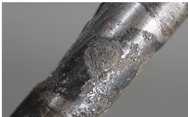
Plate 3: Dissimilar metal corrosion.
