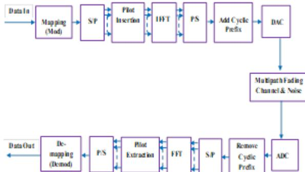
Fig. 1 Conventional OFDM System Model
