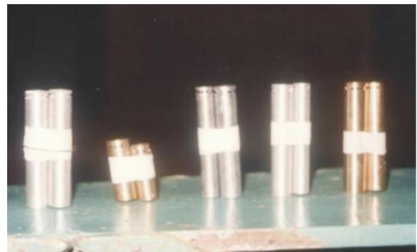
Fig. 1: Casted and Machined Anodes Produced Locally
