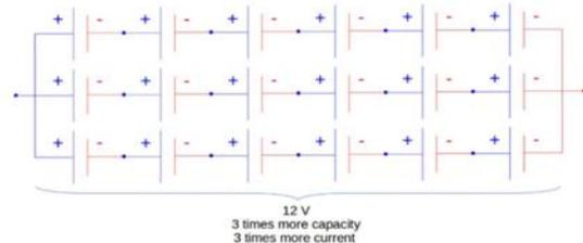
When the cells are connected in parallel the voltage magnitude remains same but the current magnitude varies with respect to the number of cells connected in the pack.
